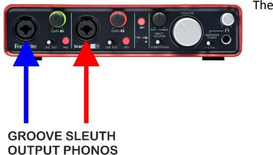
The Groove Sleuth Mk.II is connected to your sound-card's line inputs (as shown above). Levels should be set on the interface in the normal way and you will find that the preamplifier delivers audio at a sufficiently high level for all commercial sound-cards, both internal and external.
