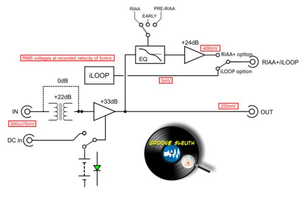
The **Groove Sleuth Mk.II** preamplifier is suitable for high-output moving-coil (HMC) and moving-magnet (MM) cartridges, and optional transformers may be fitted for low-output moving-coil (MC) cartridges. The **Groove Sleuth Mk.II** is also suitable for Phaedrus Audio **PHLUX (PHLUX II)** active moving-magnet cartridges. (See Chapter 5 for more information about **PHLUX** active cartridges.)
