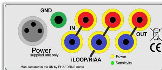
In the base options, the unit simply presents the cartridge with the correct impedance at the IN phonos and amplifies the signal. The output is presented on the phonos marked OUTPUT on the rear of the **Groove Sleuth Mk.II** unit.
