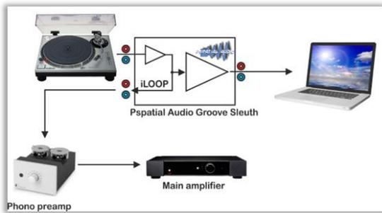
The **Groove Sleuth Mk.II** preamplifier features the **iLOOP**; a wide-bandwidth, low-noise and distortion buffered loop-through. This is especially convenient for enthusiasts who already have an excellent LP replay solution but who want to introduce computer audio into their system. This is because the **Groove Sleuth Mk.II** integrates transparently into a pre-existing setup and provides new functionality without upsetting what's there already.
