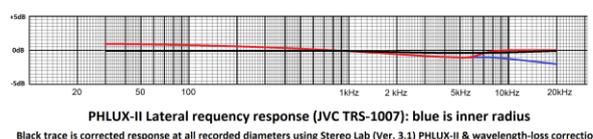
The PHLUX-II cartridge has a very level frequency response. Variation is confined to  $\pm 1$ dB. This is a very good result and is illustrated in the graph above by the red trace.
